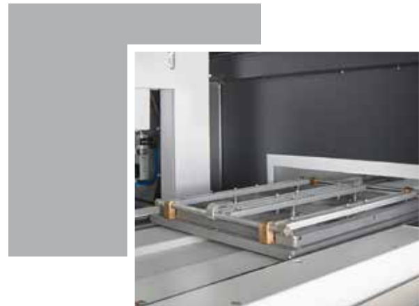
View on the transfer of the carrier from the lifting station to the conveyor belt.
