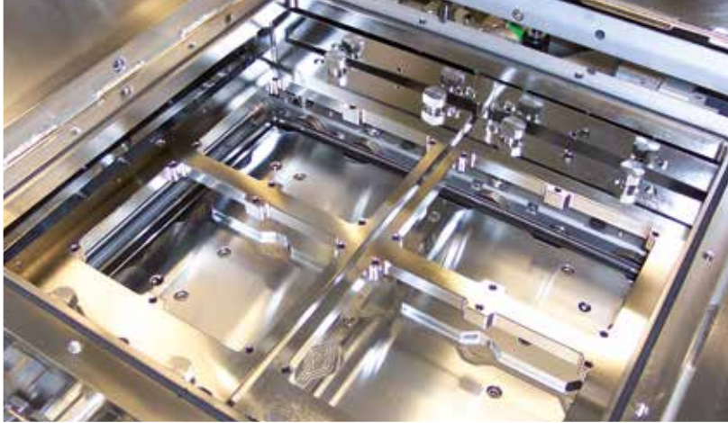
Carrier with integrated downholder frame for automatic fixture in the process chamber.
